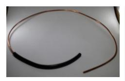
Slide half of the rubber over one end of the bare copper, as shown below.
